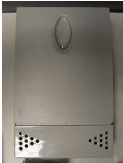
The OEM combined temperature and RH sensor
